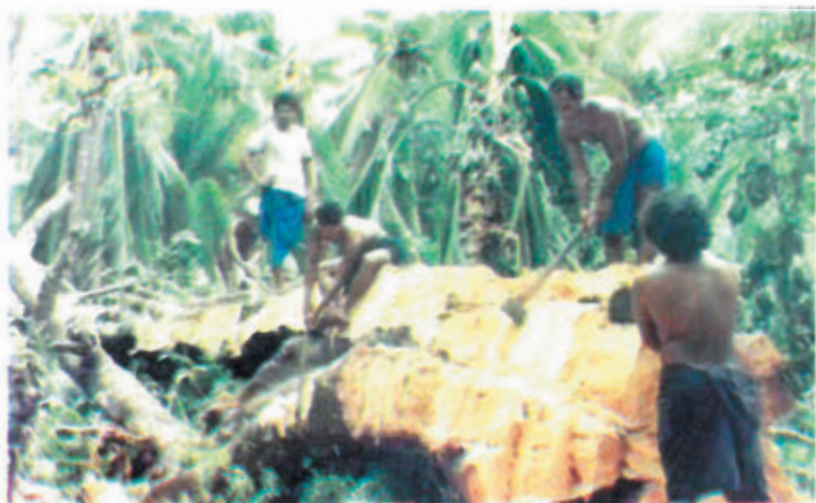
Men from Satawal shaping a breadfruit tree trunk that will be used to make the hull of a sailing canoe.
