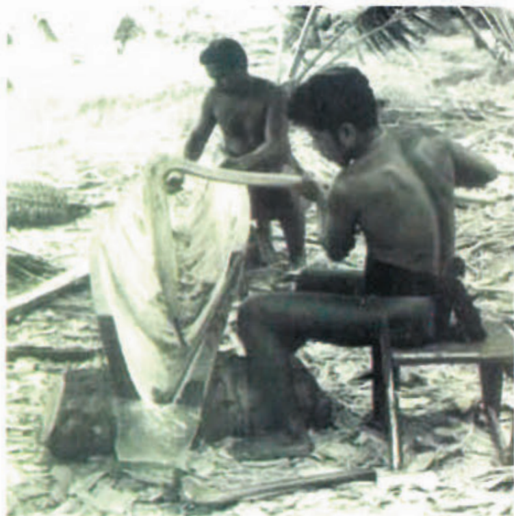
Tihwe of Satawal uses a special adze to shape the hull of a small canoe while Tereyong works on the mas (eye of the canoe). This photo was taken in the early 1970s.
